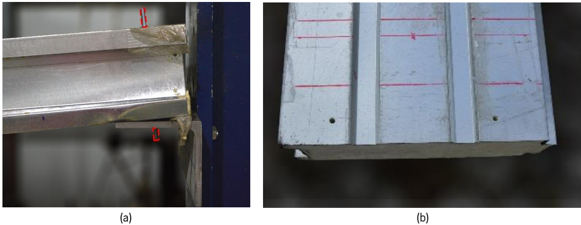
Figure 6.30. Failure progression and inspection after the flexural test of connection system 1L: (a) tilting of the bolts at the end of the test; (b) undamaged bolt holes after disassembly.
