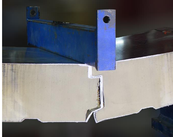
Figure 6.15. Tensile cohesive failure of the PUR foam near the face sheet-to-core interface.
