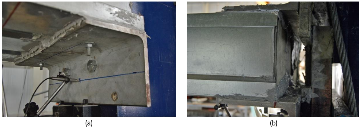
Figure 6.33. Support conditions of specimen 2LA-01: (a) adhesive excess in the bottom steel angle; (b) adhesive spill in the end cross-section of the sandwich panel.
