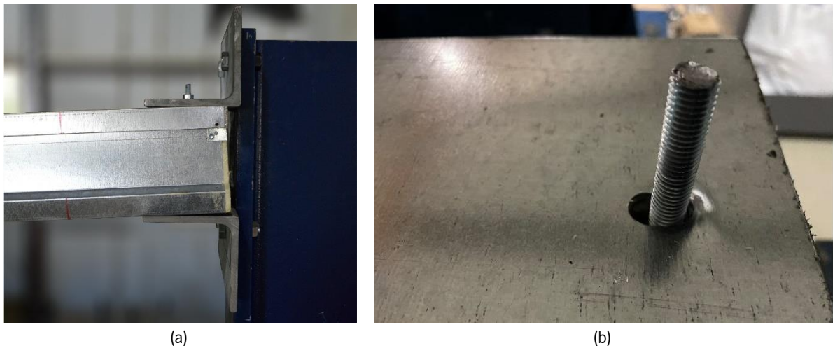
Figure 6.32. Inspection after the flexural test of connection system 2L: (a) rotation at the support; (b) bearing failure of the bolt holes after disassembly.
