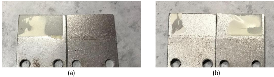
Figure 4.27. Observed failure modes in the single lap shear test: (a) SLST-02; (b) SLST-04.
