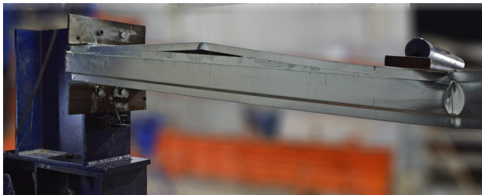
Figure 6.36. Debond between the top plain C-section and bottom lipped C-section of the sandwich panel.
