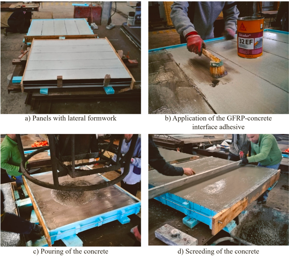
Fig. 5. Preparation of the hybrid sandwich panel.
