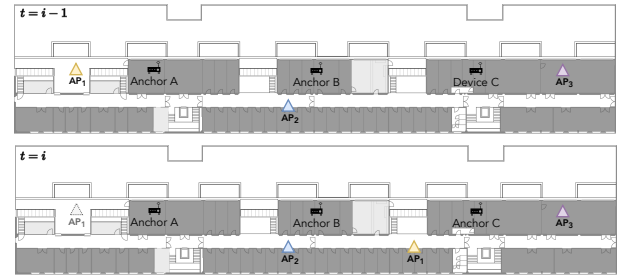
Fig. 3: AP position change between two time instants.
