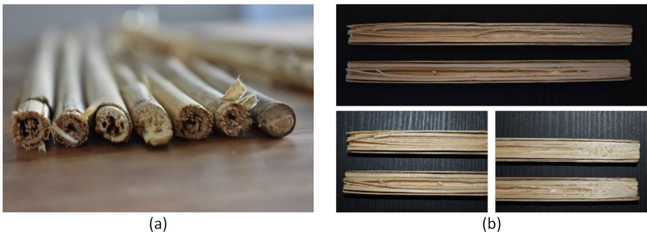
Fig. 2 Cortaderia selloana stems. (a) Cross-section on various parts. (b) Longitudinal section
