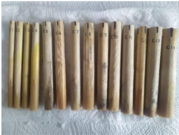
Fig. 4 Group C samples after 96 h on water absorption by capillarity test
