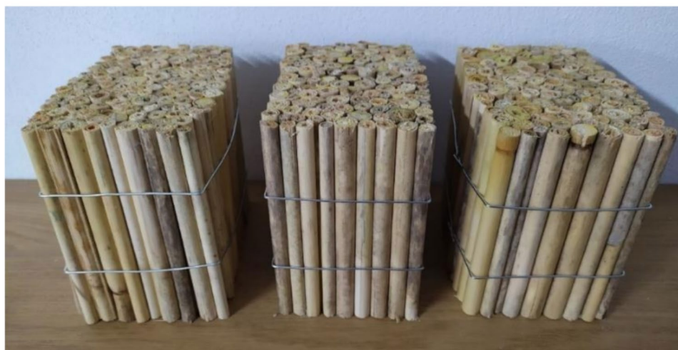
Fig. 12 Cortaderia Selloana insulation panel with entire stems
