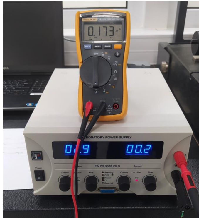
Figure 34 - Power supply assembled with a multimeter
