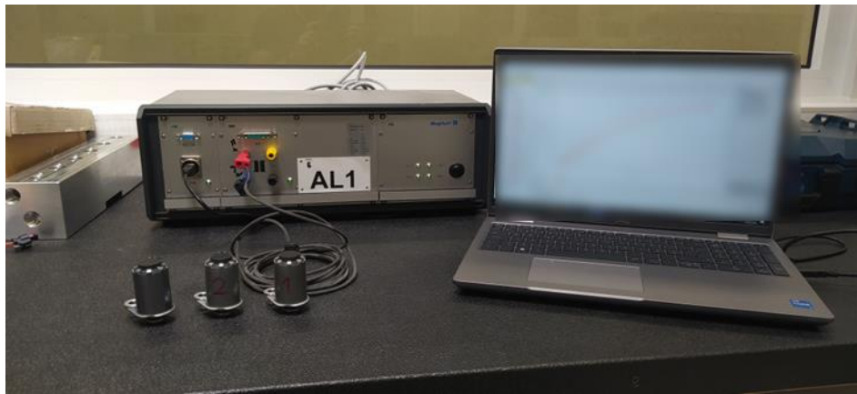
Figure 38 – Magnetic flux testing of the solenoid valves in the MagHyst
