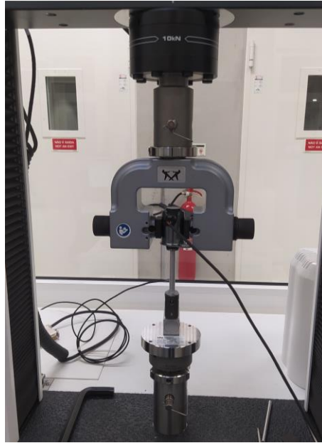
Figure 35 – Mounting of the solenoid valve for the measurement of magnetic force
