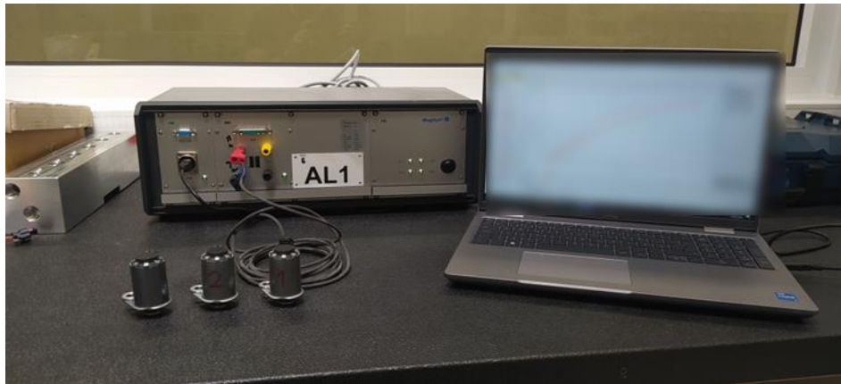
Figure 36 - Magnetic measurements for solenoid valves with MagHyst
