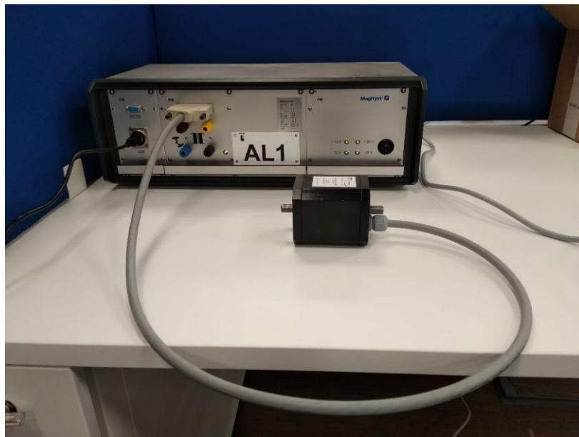
Figure 24 - MagHyst modular and rod adapter mounted for testing
