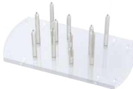
(c) The 11 target stalks of the phantom box.
