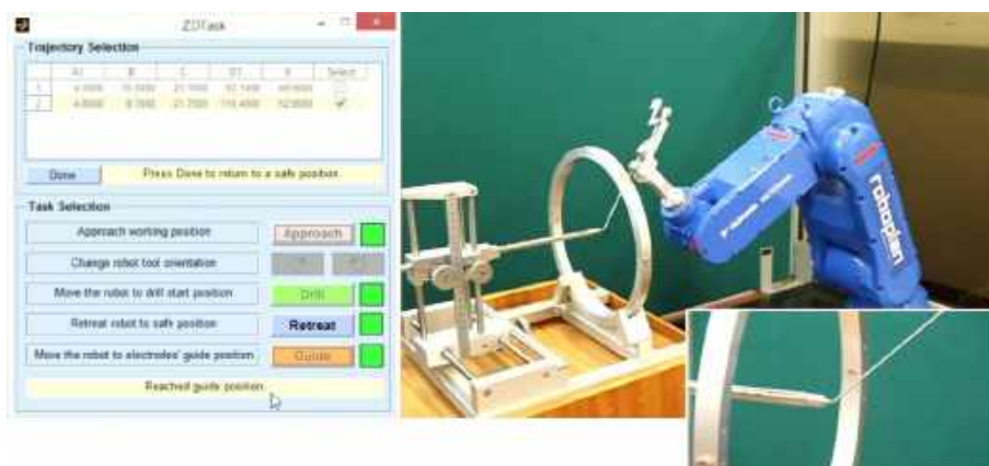
Figure 4.10: Holding microdrive to position electrode at the surgical target.
