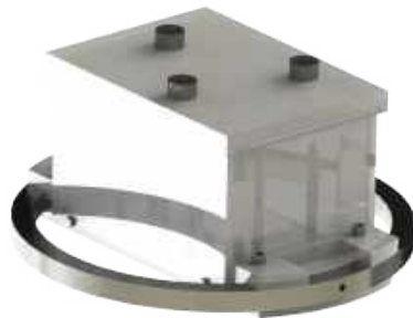
(b) Closed phantom with 3 female interlocks used for registration.
