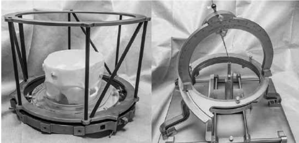
Figure 2.2: BRW “N-pattern” localizer and stereotactic frame mounted on a “phantom-base” verification device (Mozdy, 2017).
