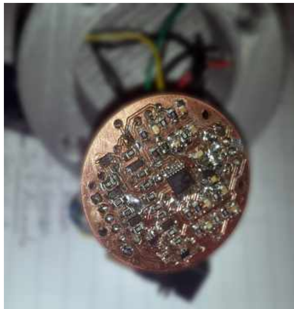
Figure 5.10: 4-button debounce PCB.
