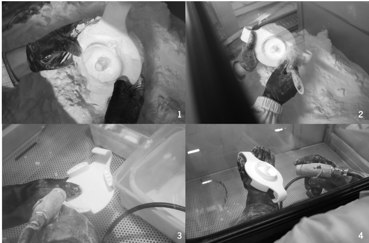
Image 29: Cleaning Process Stages 1 - Unpacking; 2 - Brush Clean-up; 3 - Compressed Air cleaning; 4 - Low Pressure Air Dusting.
