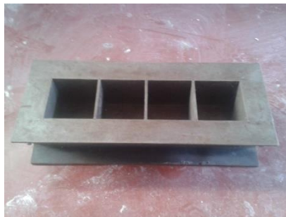
Figura 20 – Molde de provetes cúbicos (100x100x100) (mm 3 )
