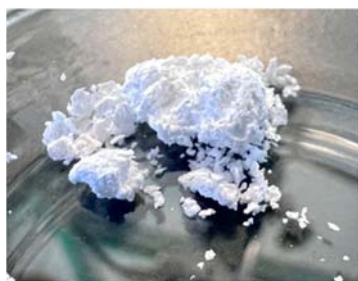
Fig. 6 Resultant PHA precipitate (dried in an oven at 60 °C for 6 hours).
