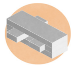
Wood-only connectors inspired by handcrafted carpentry and cabinet-making
