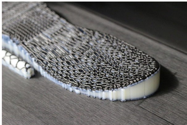
FIG. 7.21 PolyJet prototype with support material. (Courtesy of DONE Lab - Advanced Manufacturing of Products and Tools , Guimarães, Portugal.)
