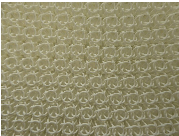
FIG. 7.28 SLS chainmail model. (Courtesy of DONE Lab - Advanced Manufacturing of Products and Tools, Guimarães, Portugal.)
