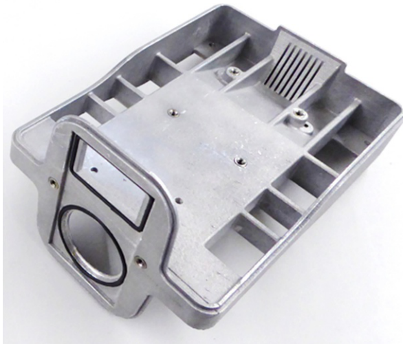
FIG. 7.32 DMLS aluminum models. (Courtesy of DONE Lab - Advanced Manufacturing of Products and Tools, Guimarães, Portugal.)
