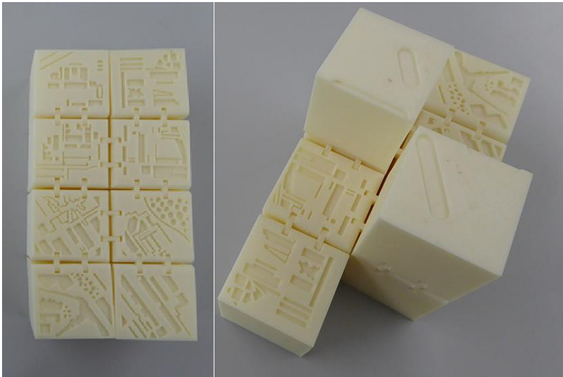
FIG. 7.18 FFF right space between moving parts. (Courtesy of DONE Lab - Advanced Manufacturing of Products and Tools, Guimarães, Portugal.)
