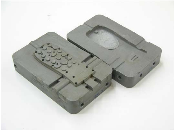
Figure 6. Core and cavity made by epoxy tooling.
