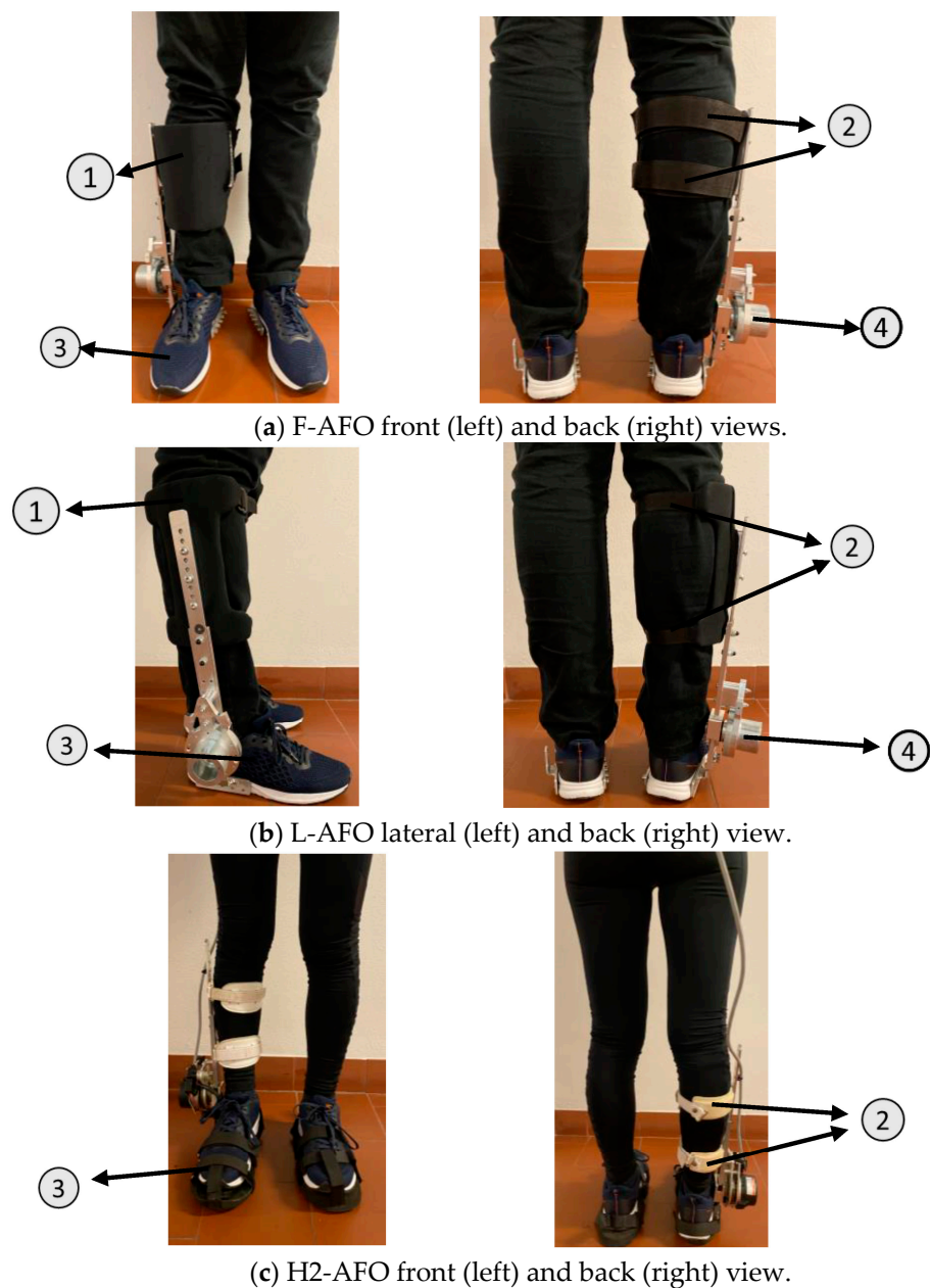
Figure 1. Representation of the modules of the three AFOs used in this study. (a) F-AFO (team-developed AFO). (b) L-AFO (team-developed AFO). (c) H2-AFO (Technaid S.L.). 1—Shin-guards. 2—Shank fixation (straps/cuffs). 3—Foot fixation. 4—Actuation structure.
