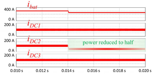
Fig. 10. Results showing the transient-state current in the EV battery ( i_{bat} ), resulted from the sum of the output current of all the DC-DC power modules ( i_{DC1} , i_{DC2} , and i_{DC3} ), demonstrating that each DC-DC power module is controlled individually, in this case, with a sudden variation of the current i_{DC2} , forcing to reduce also the current in the EV battery ( i_{bat} ).
