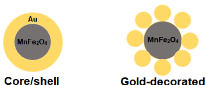
Figure 1.9. Schematic representation of the nanoparticles studied in this work, the manganese ferrite/gold core/shell nanoparticles and the gold-decorated manganese ferrite nanoparticles.
