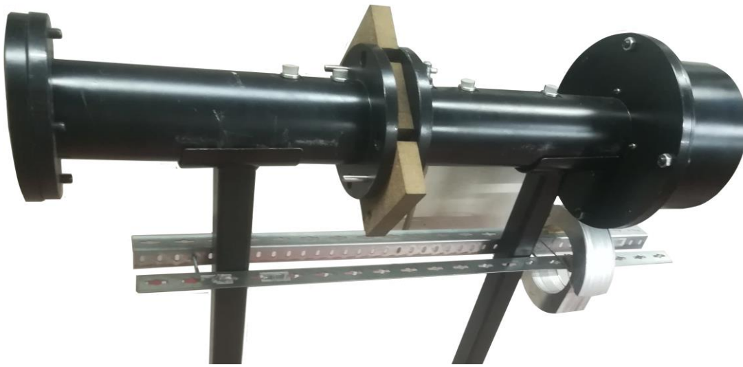
Figure 6.7. Detail of impedance tube assembly for Transmission loss testing.
