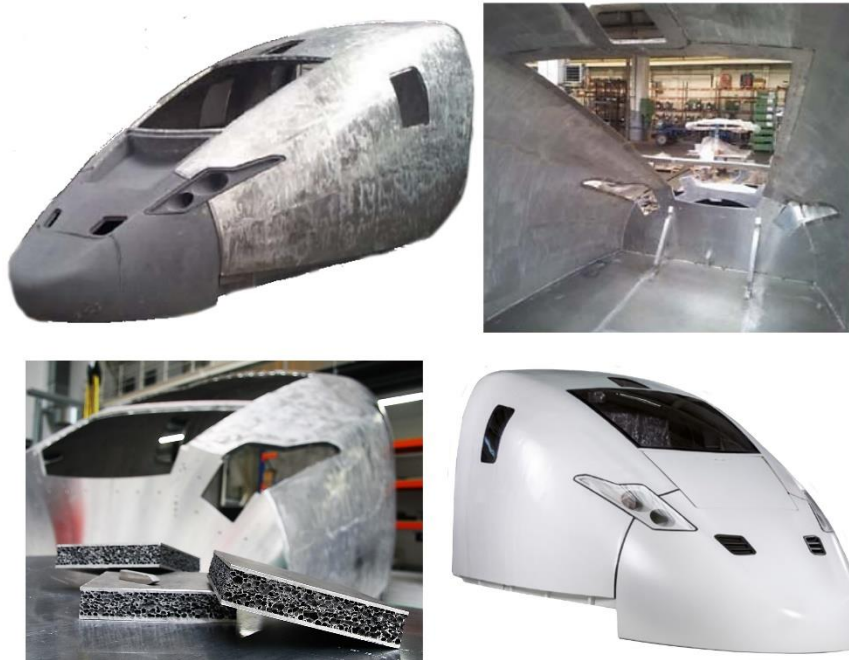
Figure 1.3 Prototype of a train front manufactured with welded cellular sandwich panels (adapted from [12,14,15]).
