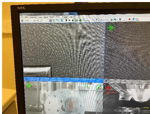
Figure 30 - topographic visualization of a sample magnified 424x in SEM
