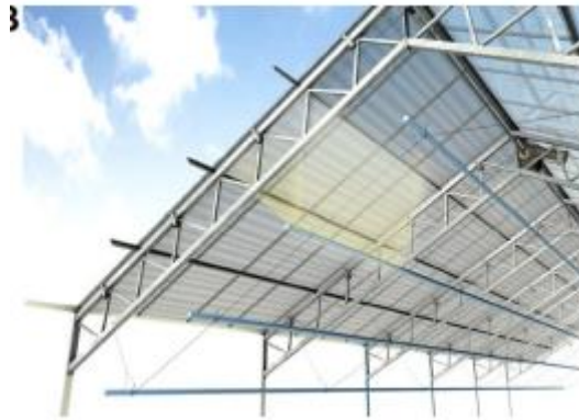
Figure 20 - Linear Fresnel lenses focusing light on a strip of a PV module taken from [27]
