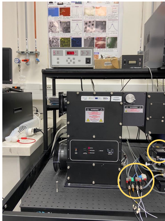
Figure 31 - Solar simulator used for the electrical measurements, at the right side we can see the 4 wires used by the 4 probes and the reference solar cell in the back
