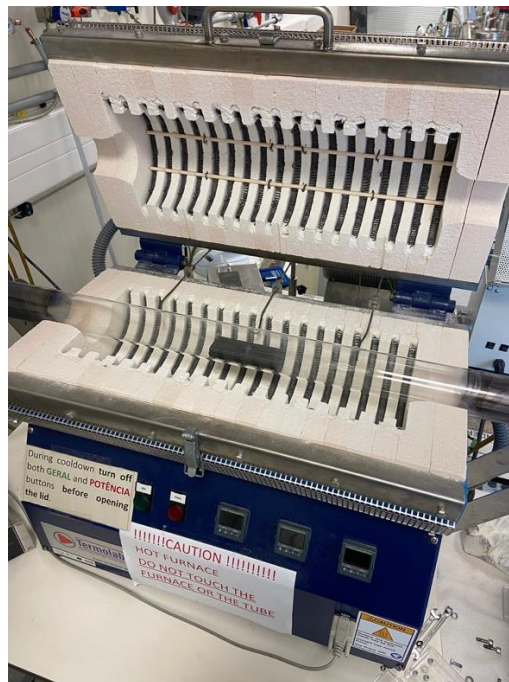
Figure 30 - Tube Furnace inside the LaNaSC group lab at INL
