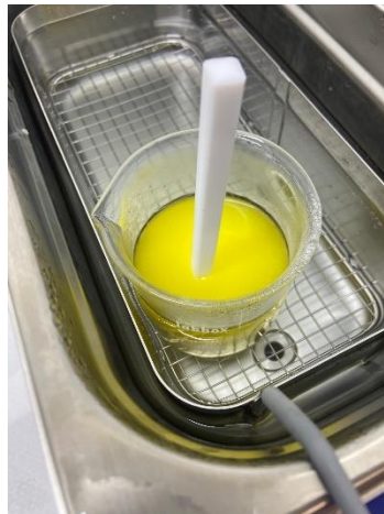
Figure 31 - Beaker containing the sample holder (white) and the solution that deposits the window layer (yellow)
