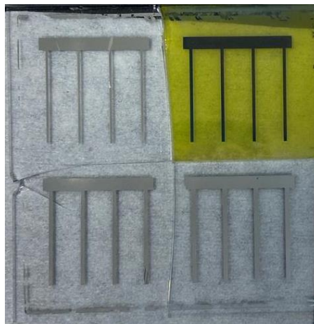
Figure 35 - Full 5 \times 5 \text{ cm}^2 sample and the 4 divided smaller sections of 2.5 \times 2.5 \text{ cm}^2
