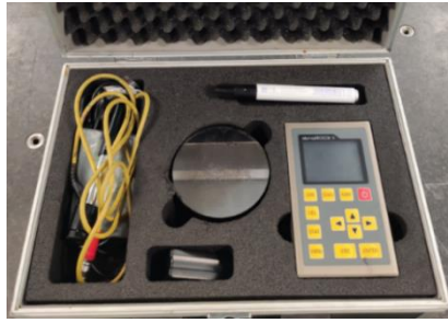
Figure 79 – BAQ dynaROCK II portable hardness measuring device.
