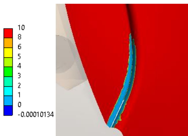
Figure 240 – Safety factor determined by the Sines method at the fitting region on the cavity side of Fat_3.
