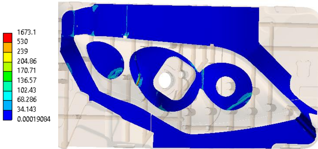
Figure 237 – Maximum alternated stress in MPa at each location by the Sines method at the fitting region on the cavity side of Fat_3.
