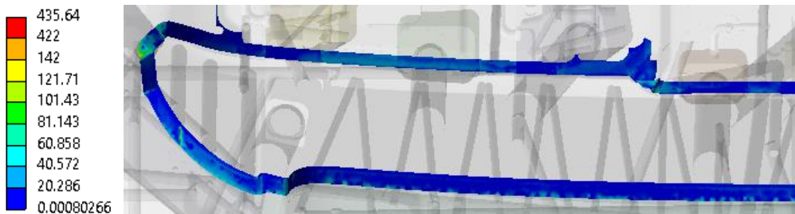
Figure 261 – Maximum alternated stress at each location by the Sines method at the fitting region on the core side of Fat_4.
