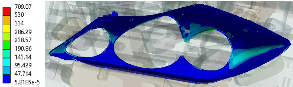
Figure 241 – Maximum alternated stress in MPa at each location by the Sines method at the core engraving region of Fat_3.
