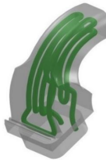
Figure 13 - Conformal cooling channels example made in one insert.
