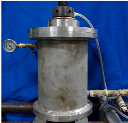
Fig. 6. Permeability test vessel.
