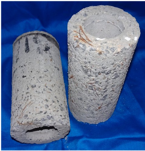
Fig. 16. Concrete flaking of hollow cylinder specimen after FT cycles.
