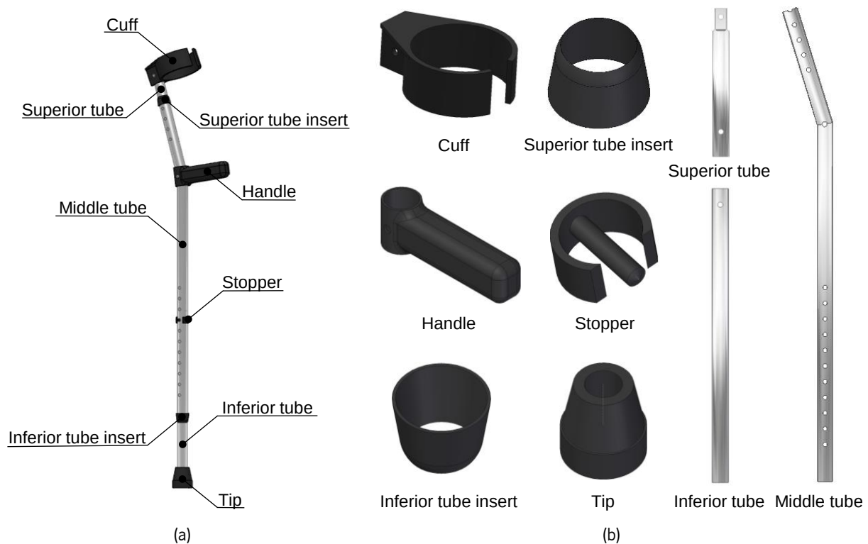
Figure 6.2 – The CAD models of the (a) C8 closed cuff crutch and (b) mechanical components. The figure is not to scale.
