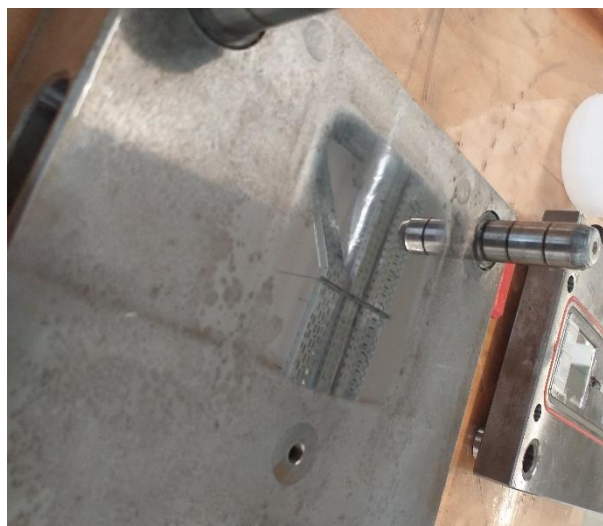
Figure 41 - Polished surface on the injection side.
