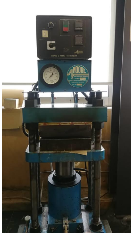
Figure 25 - Improvised hot embossing station from a hydraulic press.
