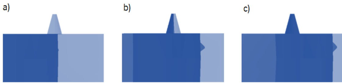
Figure 66 – Flow behaviour in microstructures filling (Molded3D simulation).
