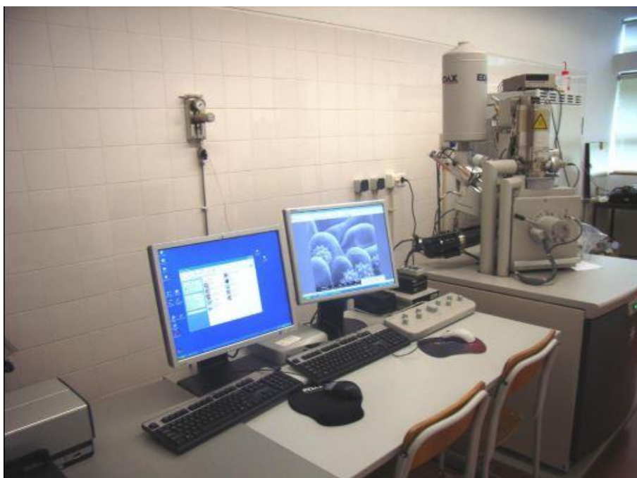
Figure 32 – SEM characterization station at SEMAT: FEI Nova 200 and EDAX Pegasus X4M equipment.
