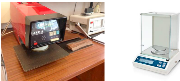
Fig. 5: Alambeta device and analytical balance for thermal and moisture absorption tests, respectively
