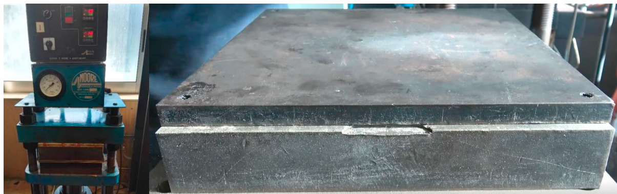
Fig. 2: Moulding compression equipment and mould used
