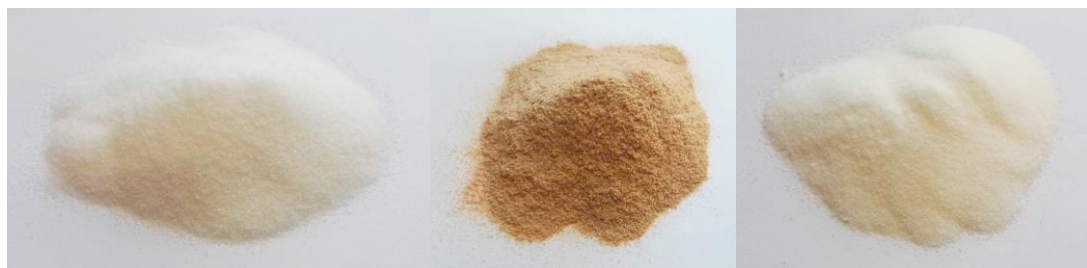
Fig. 1: Raw-materials, namely PP, wood powder and MAPP, respectively
