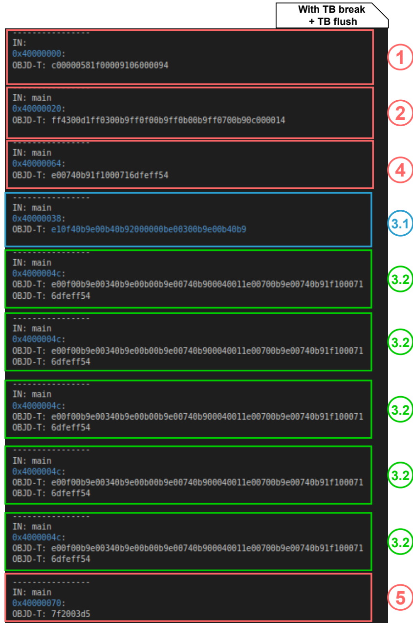
Figure 4.1.11: Log output for TB flushing and brekaing.
