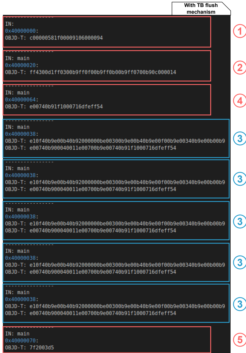
Figure 4.1.10: QEMU logs result with active TB flush mechanism.
