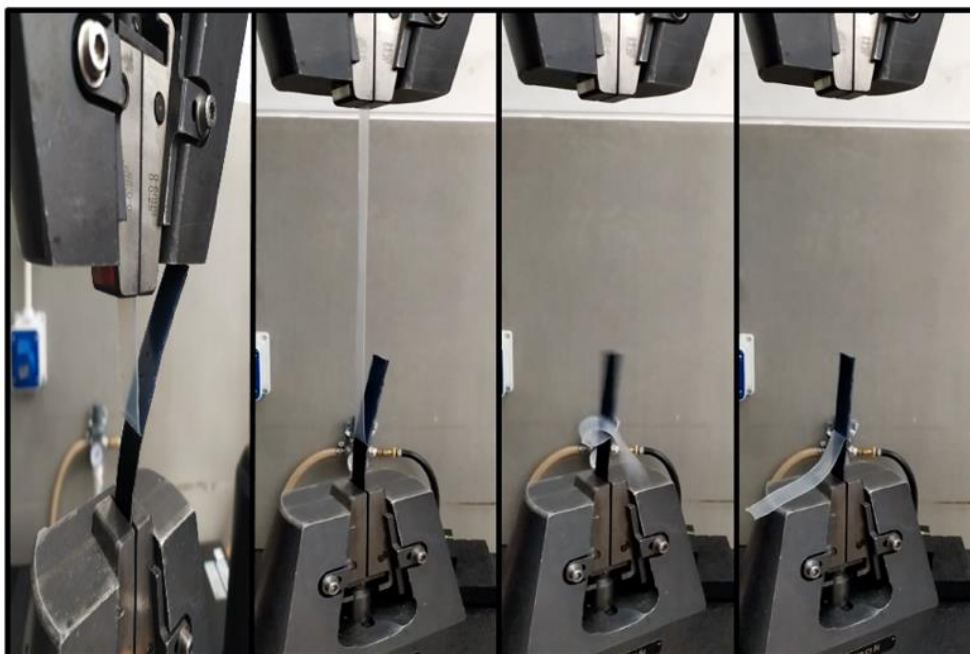
Figura 49. Peel test PC/ABS com TPU
