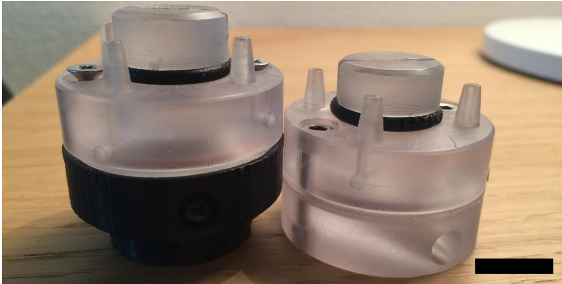
Figure 7.2 | Perspective picture of the dual-chambers. On the left, the dual-chamber is attached to the bottom part designed to attach in the newest version of the dynamic platform. On the right the dual chamber is attached to the bottom part which fits a commercial 6-well plate (scale bar = 10 mm).
