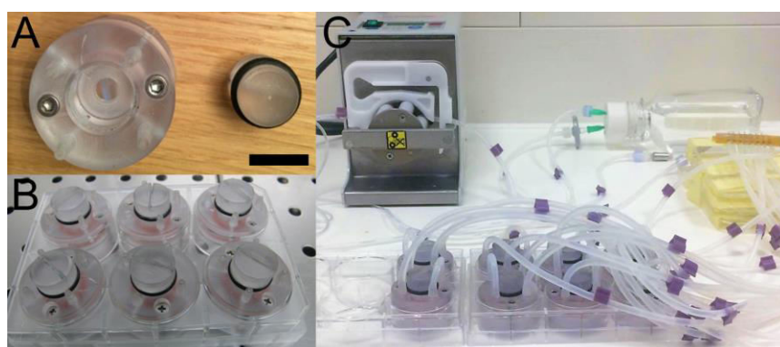
Figure 6.1 | Dual-chambers. (A) Top view of a dual-chamber with opened top and top cap on the right side, turned down (scale bar = 15 cm). (B) Dual-chambers placed in a commercial 6-well plate. (C) Dual-chamber bioreactor system assembled for flow perfusion.
