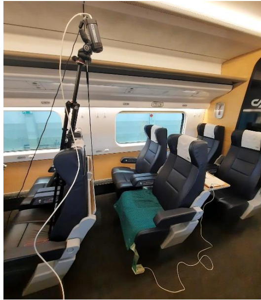
Figure 6.4. Experimental setup developed to assess the pressure and temperature at the seat-passenger interface.
