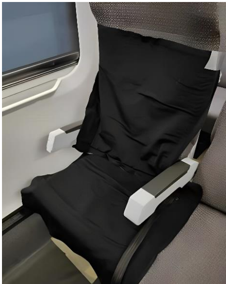
Figure 2.7. Interface pressure experiments (a) typical body pressure distribution (adapted from [59]); (b) experimental setup employed by Peng et al. on a Chinese high-speed rail 2nd class seat (adapted from [62]).
