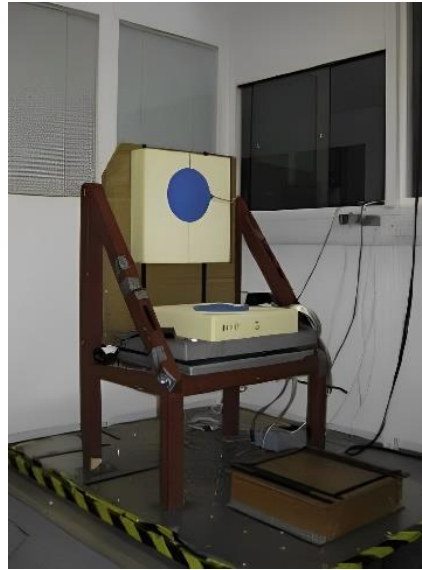
Figure 2.4. Transmissibility experimental setup used in laboratory experiments with seat simplification. (Adapted from [48]).
