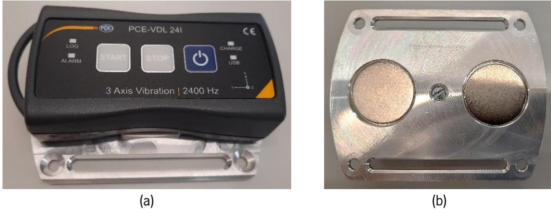
Figure 3.1. 3-axial accelerometer attached on the mounting plate where (a) top view and (b) bottom view.
