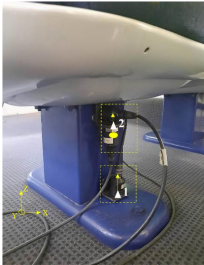
Figure 5.16. Experimental setup: (a) seat pad location; (b) accelerometers on seat frame structure.
