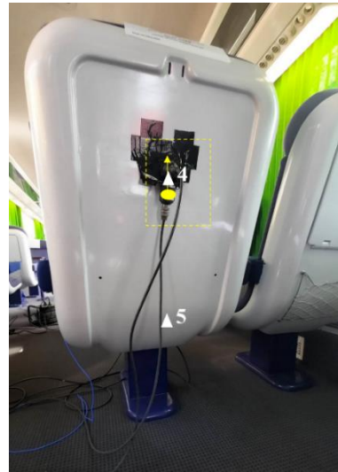
Figure 5.16. Experimental setup: (a) seat pad location; (b) accelerometers on seat frame structure.
