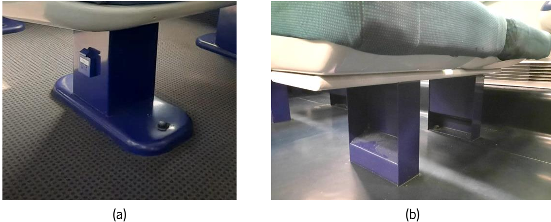
Figure 5.15. Seat metallic structural frame: (a) comfort seat structural frame; (b) standard seat structural frame.
