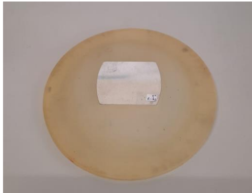
Figure 3.4. Developed system, metallic box coupled with a silicone rubber 80 Shore A disc.
