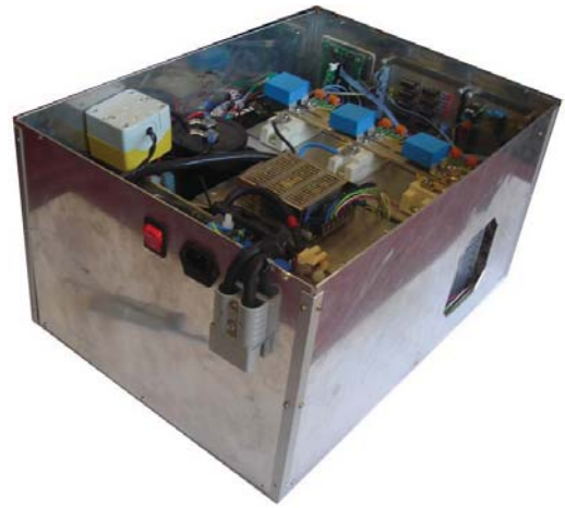
Figure 12. External view of the developed laboratory prototype of the Smart Batteries Charging System of the Electric Vehicle CEPIUM.
