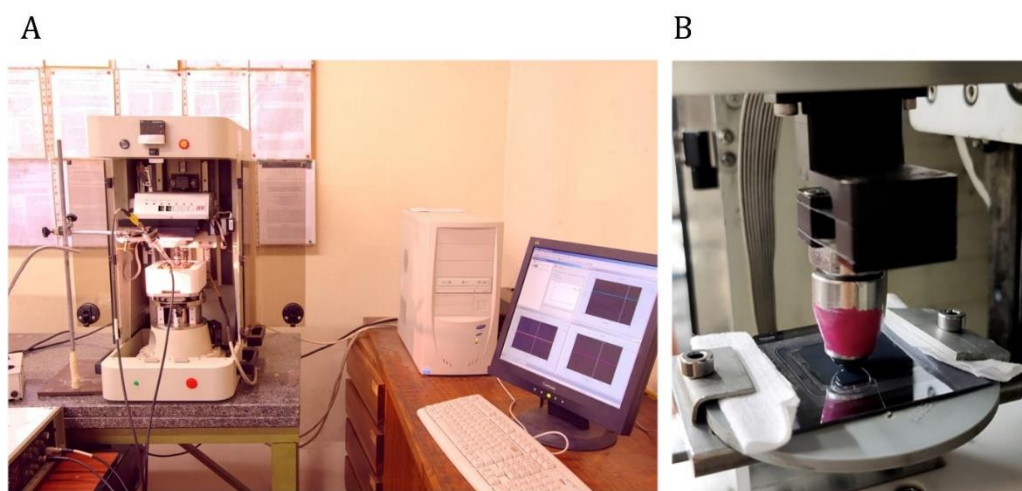
Figure 5.1 - (A) CETR-UMT2 tribometer utilized for testing and (B) Sample positioned on the tribometer for testing.
