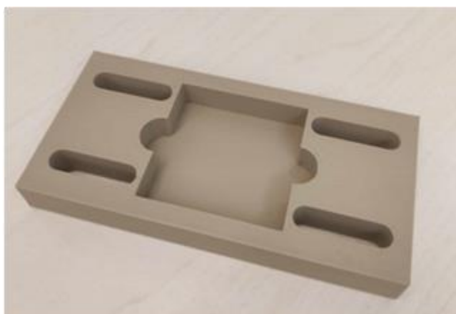
Figure 5.2 – Design of the sample support used in this work, obtained by 3D printing,
