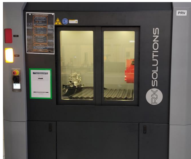
Figure 42: RX Solutions Easytom CT scanner performing x-ray projection on the pump.
