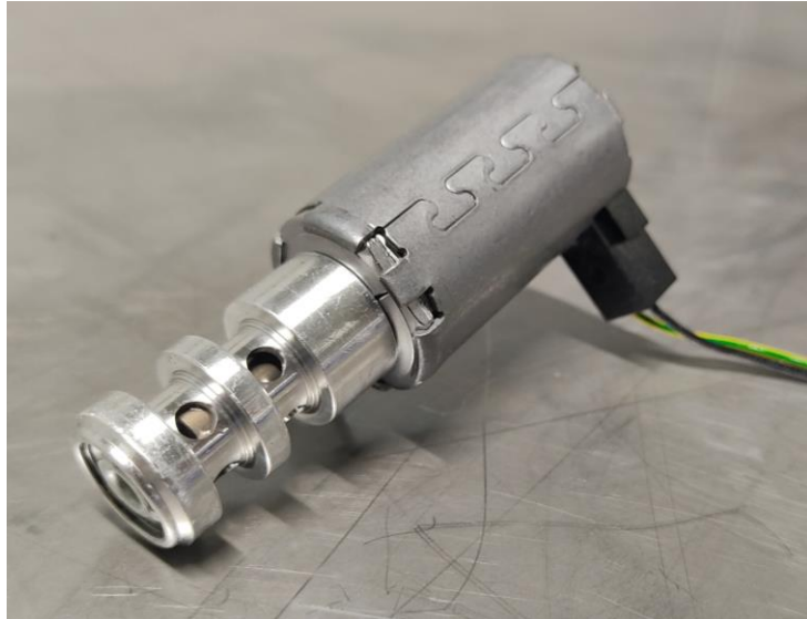
Figure 49: Solenoid valve after last crimping operation.
