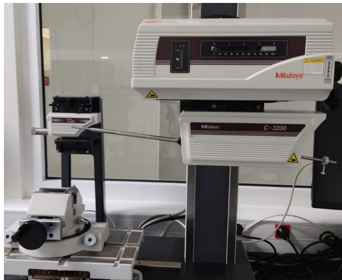
Figure 69: Mitutoyo Contracer SV-C-3200 profilometer.
