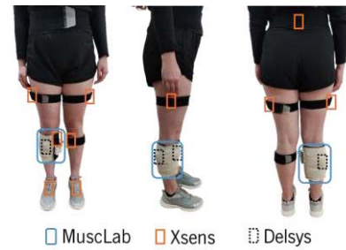
Fig. 4. Participant instrumented with the MuscLab, Delsys, and Xsens systems.
