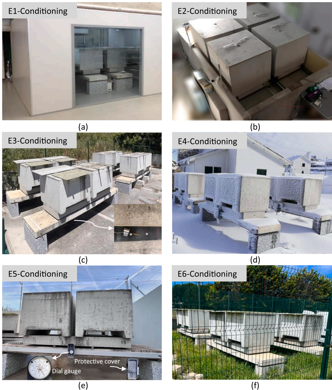
Fig. 3. Environmental exposures: laboratory-based with (a) conditioning at 20 °C and 55 % relative humidity; (b) conditioning at 20 °C under tap water immersion; outdoor environments mainly promoting degradation due to (c) high CO 2 emissions, (d) freeze-thaw attacks, (e) high temperatures, and (f) high humidity and airborne chlorides.
