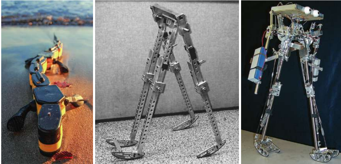
Figure 1: Examples of bioinspired robots. Left: Salamandra Robotica [Crespi et al., 2013]; Center: Reproduction [Collins et al., 2001] of the 2D gravity-powered passive design introduced by McGeer [1990]; Right: Self-powered Cornell's 3D passive dynamic walker [Collins & Ruina, 2005]
