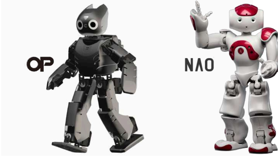
Figure 8: Humanoid platforms employed in this work. Left: Robotis OP 1 (formerly DARwIn-OP) [ROBOTIS, 2019]; Right: Softbank Robotics NAO V5 [Robotics, 2019]. Refer to Appendix B: Humanoid Platforms for detailed information about both robots.
