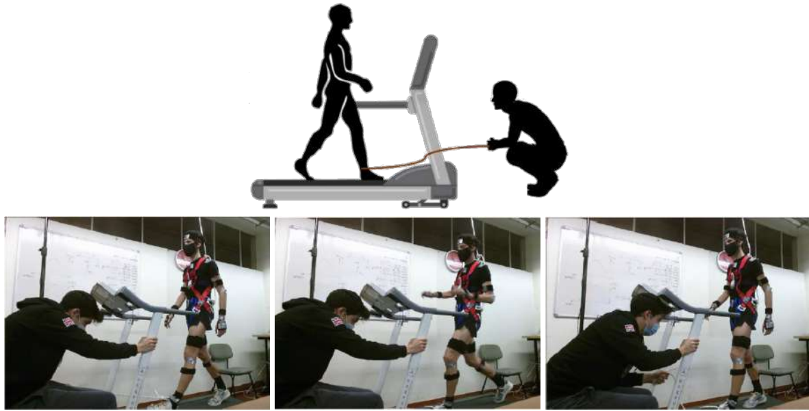
Figure 37: Experimental apparatus ( Top ) adopted in the human walking trials, with brief snapshots of a perturbation being induced by the operator ( Bottom ). Adapted from [Ferreira, 2022].
