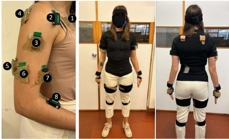
Figure 49: Participant instrumented with the sEMG sensors ( Trigno Avanti ®) on: 1) PECM, 2) DELTA, 3) DELTM, 4) DELTP, 5) TRILON, 6) TRILAT, 7) BIC, and 8) BRR ( Left ); and the inertial motion capture system ( MVN Awinda ®) in addition to the sEMG sensors ( Center, Right ).
