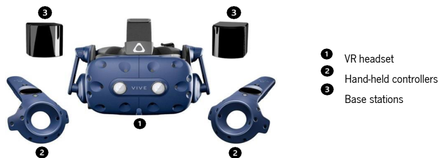
Figure 3.1 - HTC Vive Pro Full Kit composed by a VR headset, two controllers, and two base stations [57].
