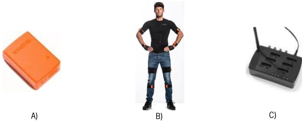
Figure 3.2 - Xsens MVN Awinda: A) MVN Wireless Motion Tracker (MTw); B) MVN Awinda MTw's position on body with adjustable straps; C) MVN Awinda station [62].
